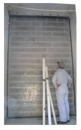
The explosive charge and standoff distance were selected to achieve the desired peak pressure and impulse on the external wall surface.
