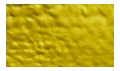
The PTS top coating shown below is an example of pinhole formation as a result of application over an improperly applied and cured sealer coating. The coating also exhibited very weak adhesion to the sealer layer.
